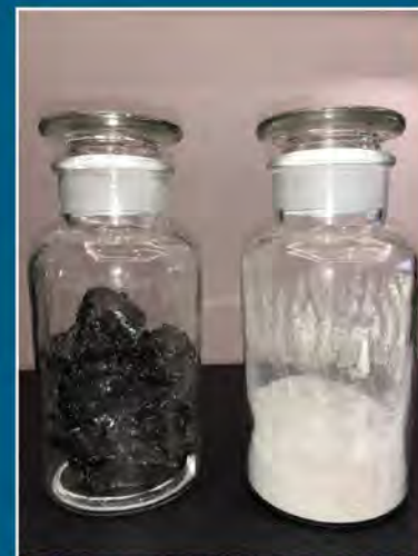
飞灰固废与熔融玻璃体 Fly ash solid waste and molten vitreous body
